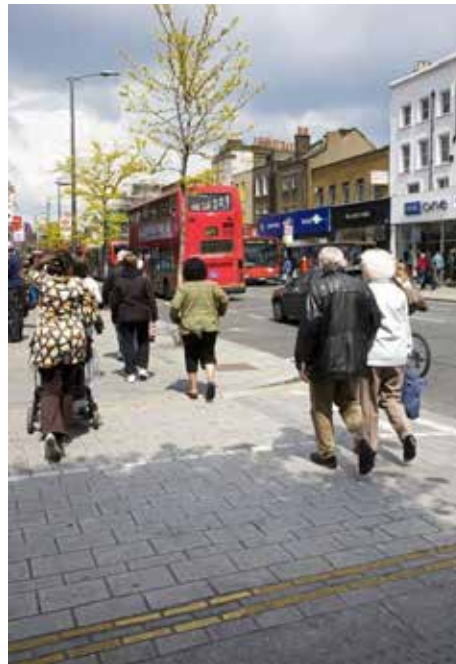
Easier pedestrian movement due to the removal of unnecessary street clutter and the creation of raised side street crossings at Walworth Road (CABE)
