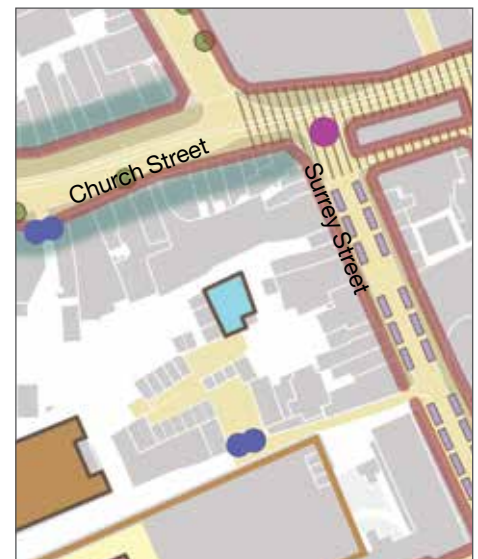
Figure 37: Blue dots on the plan indicate where boundary treatment should be considered for alleyways. Gates should be considered at entrances to private land (see page 41 for full key)
