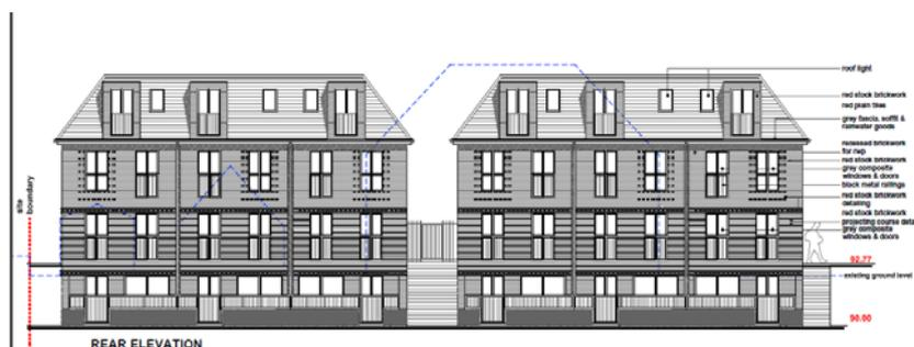
Figure 3 Proposed rear elevation showing lower ground floor
